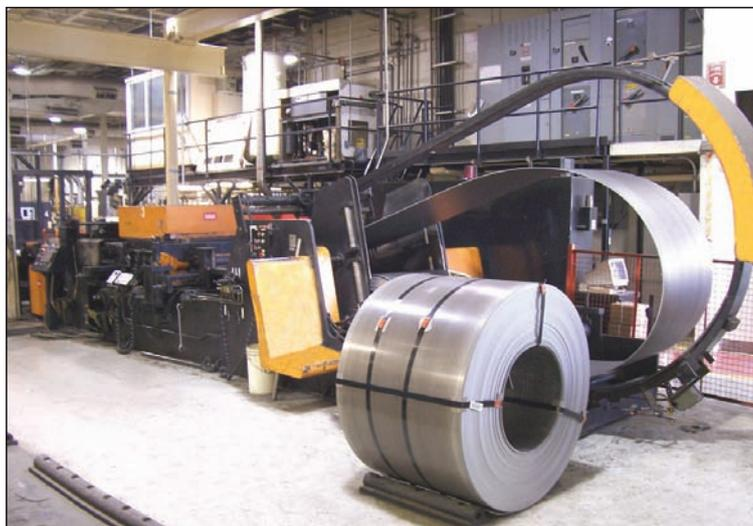
Right **Compact Coil System** allows for back load of coils directly into the cradle section.
