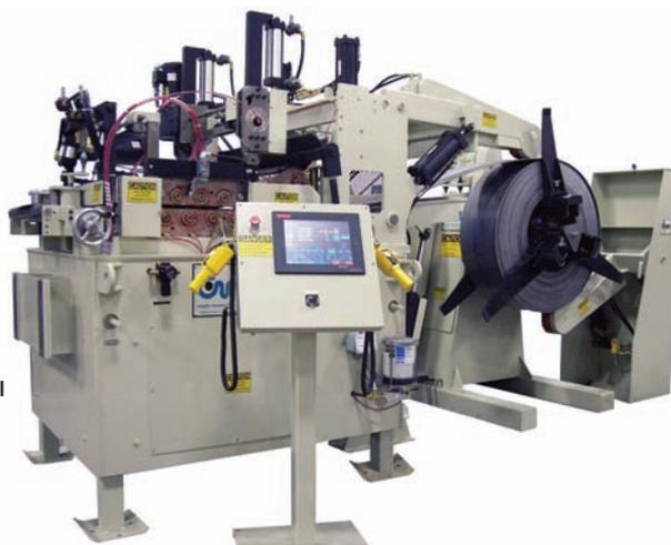
For short run, partial coil operations, Formtek has designed a compact system to handle 609 mm x 6.35 mm x 4,535.90kgs. The CWP system features a motorized uncoiler with photo eye loop control to allow the slack material to develop directly below the uncoiler spindle. Both primary and secondary hold-down arms are provided with powered rider rolls for thread-up and to allow for rewinding the slack material during partial coil operation.
